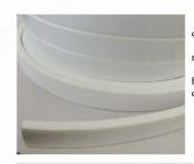
Operating temperature: -200 to +650°C; Operating pressure: 10 MPa; pH: 0-14 Sealing tape made of microwave PTFE is used for sealing flanges and connecting parts of pipelines, connecting flanges of fittings, machines, instruments, apparatuses and tanks. Field of application: gas, petrochemical, chemical, oil refining industry, engineering, medical, food and other branches of industry.
