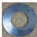
Flanged gaskets on a steel waved base (PVF) represent a flat ring with concentrically arranged undulating projections and valleys. The base profile as well as the thickness and density of the coatings are matched to each other in such a way as to ensure that the crests of the waves overlap by 0.1-0.2 mm in a compressed state at the usual specific pressure.
