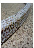
Main components: kynol fibers impregnated with PTFE suspension.
