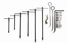
Intended use: extractors are intended for removal of wasted packing glands from stiffing boxes of fittings and pumps. The use of the extractor will allow, when removing the seal, to exclude damage to the surface of the chamber and the stem. In cases of emergency replacement of a packing gland, partial disassembly of the valve or pump is possible.
